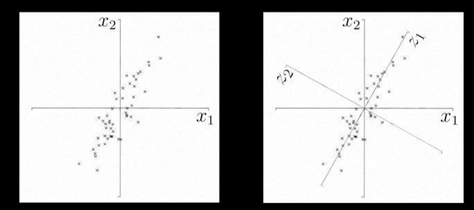
the 1<sup>st</sup> PC Z<sub>1</sub> is a minimum distance fit to a line in x space
