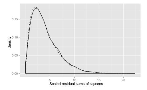
Figure 2.4: Empirical density plot of the scaled residual sums of squares, RSSsq, from simulated responses. The overlaid dashed line is the density of a  $\chi_4^2$  random variable. The peak of the empirical density gets shifted a bit to the right because of the way the empirical density if calculated. It uses a symmetric kernel which is not a good choice for a skewed density like this.
