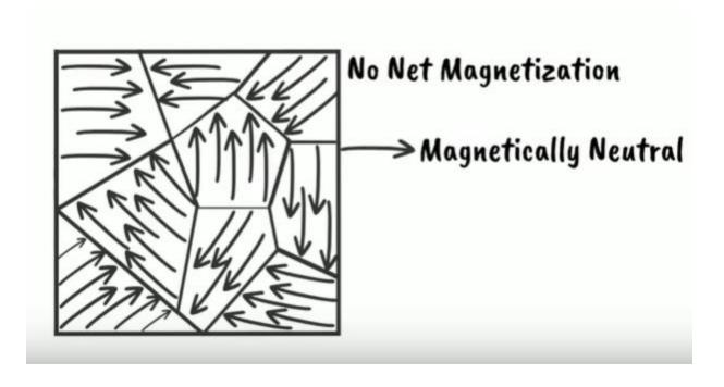
In external magnetic field magnetic domain arranged themselves in the direction of applied magnetic field hence iron becomes magnetized.
