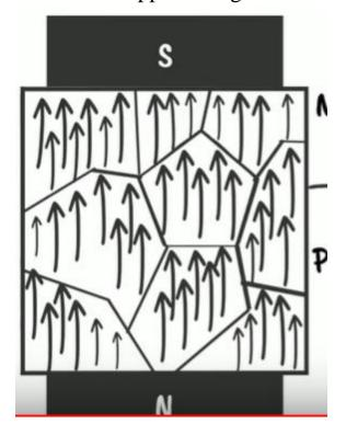
When external magnetic field is removed, it remains magnetized up to some extent. This behavior of iron is called ferromagnetism.
