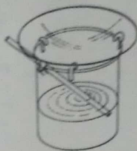
FIGURE 21.40 Arrangement for the evaporation of liquids.
