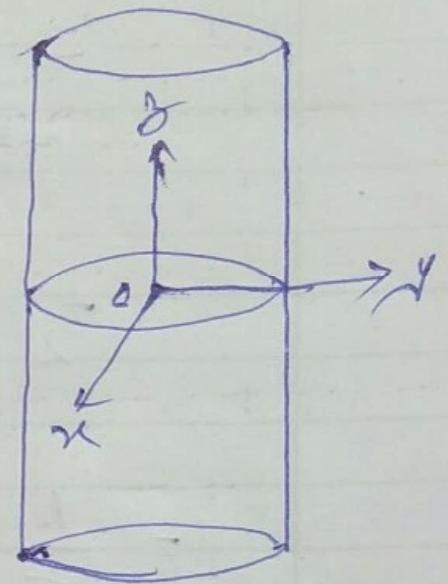
Let  $a$  is radius and  $h$  height of the cylinder. Axis of the cylinder be taken along  $z$ -axis, so that we have to find  $I_{zz}$ . Let  $O$  be taken as origin at the mid of the cylinder (c.m.)
