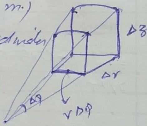
Since cylindrical coordinates are  $x = r \cos \theta$ ,  $y = r \sin \theta$ ,  $z = z$ . So moment of inertia is given by
