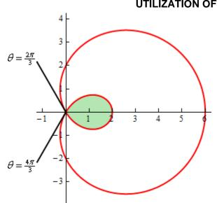
The polar curves are used to determine the mean horizontal candle power (m.h.c.p.) and mean spherical candle power (m.s.c.p.). these are also used to determine the actual illumination of a surface by employing the candle power in that particular direction as read from the vertical polar curve in the illumination calculations.
