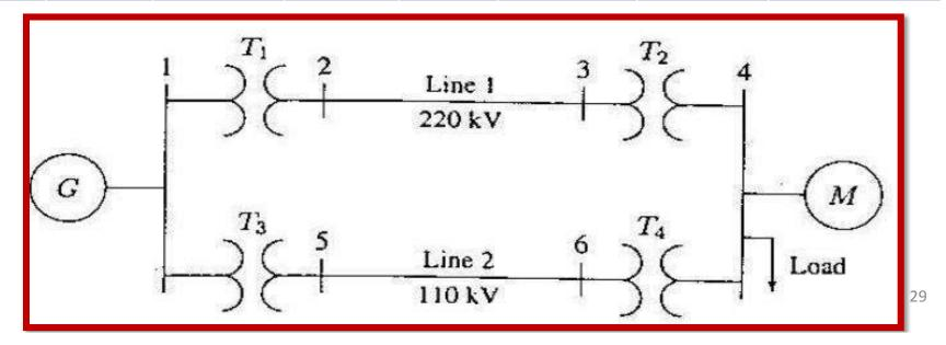
The reactance is given in percent. Its per unit is obtained by dividing it by **Solution:** 100. such as 18% = 18/100 = 0.18p.u
