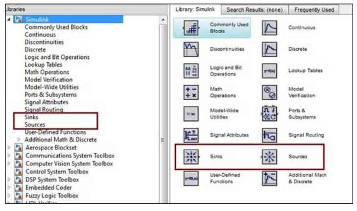
Begin by dragging the required blocks from the library to the project window. Then, connect the blocks together which can be done by dragging connectors from connection points on one block to those of another.
