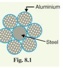
of aluminium. The result of this composite conductor is that steel core takes greater percentage of
