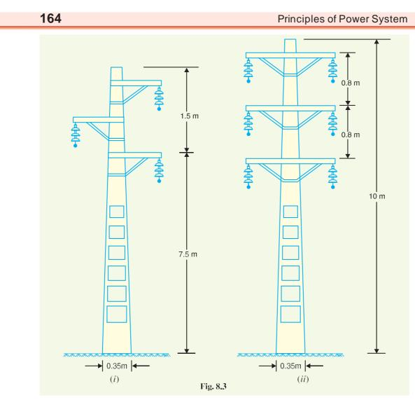
life, can withstand most severe climatic conditions and permit the use of longer spans. The risk of interrupted serivce due to broken or punctured insulation is considerably reduced owing to longer spans. Tower footings are usually grounded by driving rods into the earth. This minimises the lightning troubles as each tower acts as a lightning conductor.
