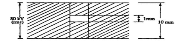
Solution: Referring to Fig. 4.5(a) and Eqs. (4.7) and (4.8), the voltage that appears across the void is given as
