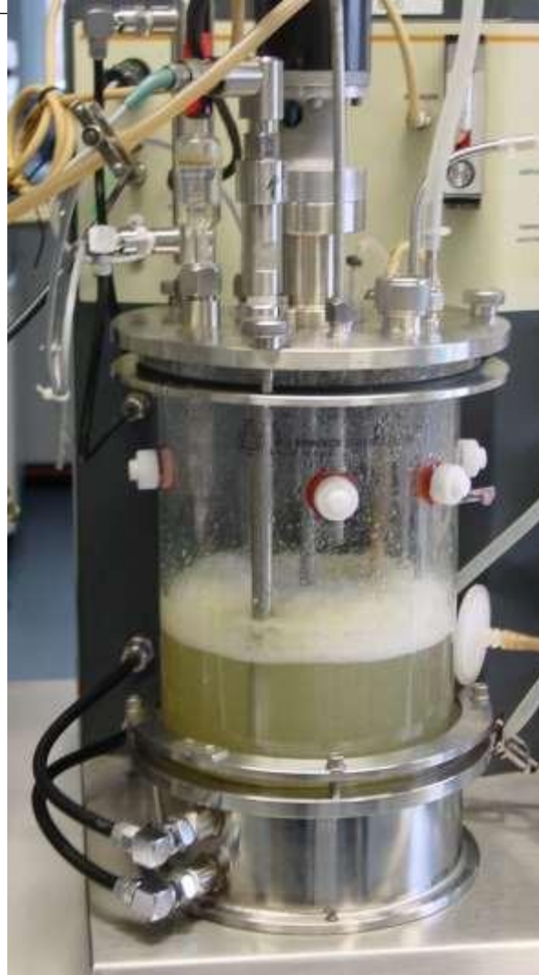
Stirred tank reactor with suspension culture of Helianthus annuus
