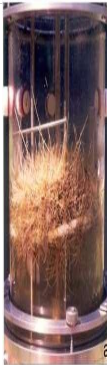
Stirred tank reactor with suspension culture of Helianthus annuus
