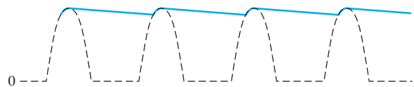
(b) Smaller ripple means more effective filtering. Generally, the larger the capacitor value, the smaller the ripple for the same input and load.
