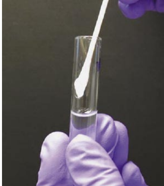
Figure 4.4 —Removing excess liquid from the swab
