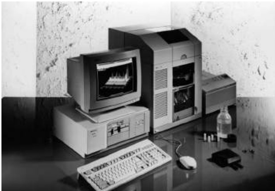
Figure 3.32. Photograph of a capillary electrophoresis system (the HP-3D capillary electrophoresis system manufactured by Hewlett-Packard). Refer to text for details. Photo courtesy of Hewlett Packard GmbH, Germany
