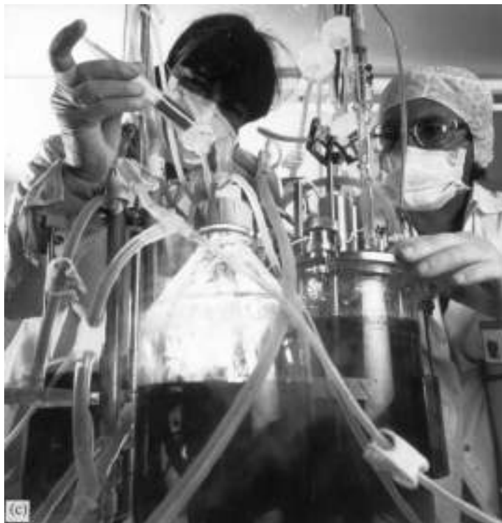
Figure 3.14. (a) Typical industrial-scale fermentation equipment as employed in the biopharmaceutical sector. (b) Control of the fermentation process is highly automated, with all fermentation parameters being adjusted by computer. (b). Photos (a) and (b) courtesy of SmithKline Beecham Biological Services, s.a., Belgium. Photo (c) illustrates the inoculation of a lab-scale fermenter with recombinant microorganisms used in the production of a commercial interferon preparation. Photo (c) courtesy of Pall Life Sciences, Ireland
