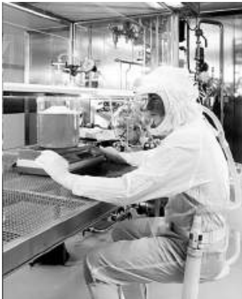
Figure 3.3. Operator wearing clean room clothing suitable for working under aseptic conditions. Note that his entire body is covered. This precludes the possibility of the operator shedding skin, microorganisms or other particulate matter into the product. Photo courtesy of SmithKline Beecham Biological Services s.a., Belgium
