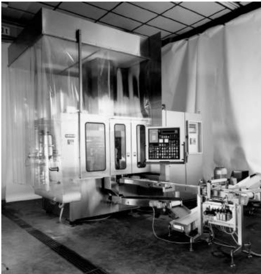
Figure 3.29. Photographic representation of a blow-fill-seal machine, which can be particularly useful in the aseptic filling of liquid products (refer to text for details). While used fairly extensively in facilities manufacturing some traditional parenteral products, this system has not yet found application in biopharmaceutical manufacture. This is due mainly to the fact that many biopharmaceutical preparations are sold not in liquid, but in freeze-dried format. Also, some proteins display a tendency to adsorb onto plastic surfaces. Photo courtesy of Rommelag a.g., Switzerland
