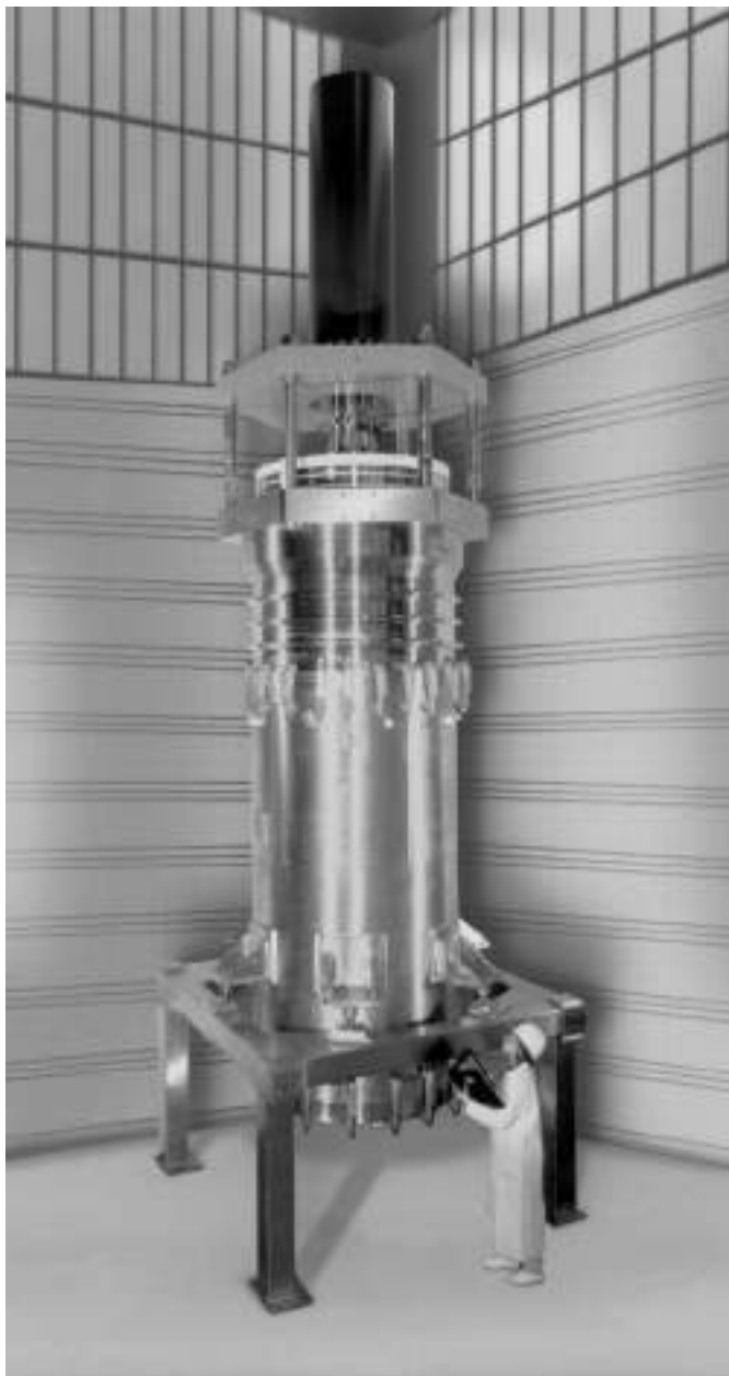
Figure 8.7. Process-scale HPLC column. Photo courtesy of NovaSep Ltd: http://www.novasep.com
