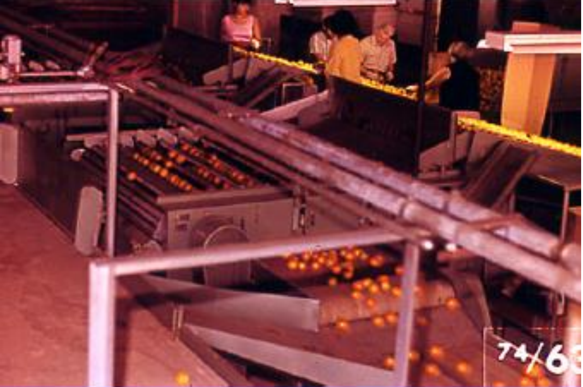
Grading for size prior to washing
