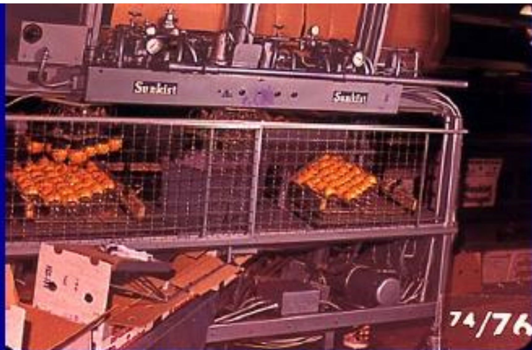
Automatic packing machine showing suction cups on the left just after they have picked up a layer of fruit
