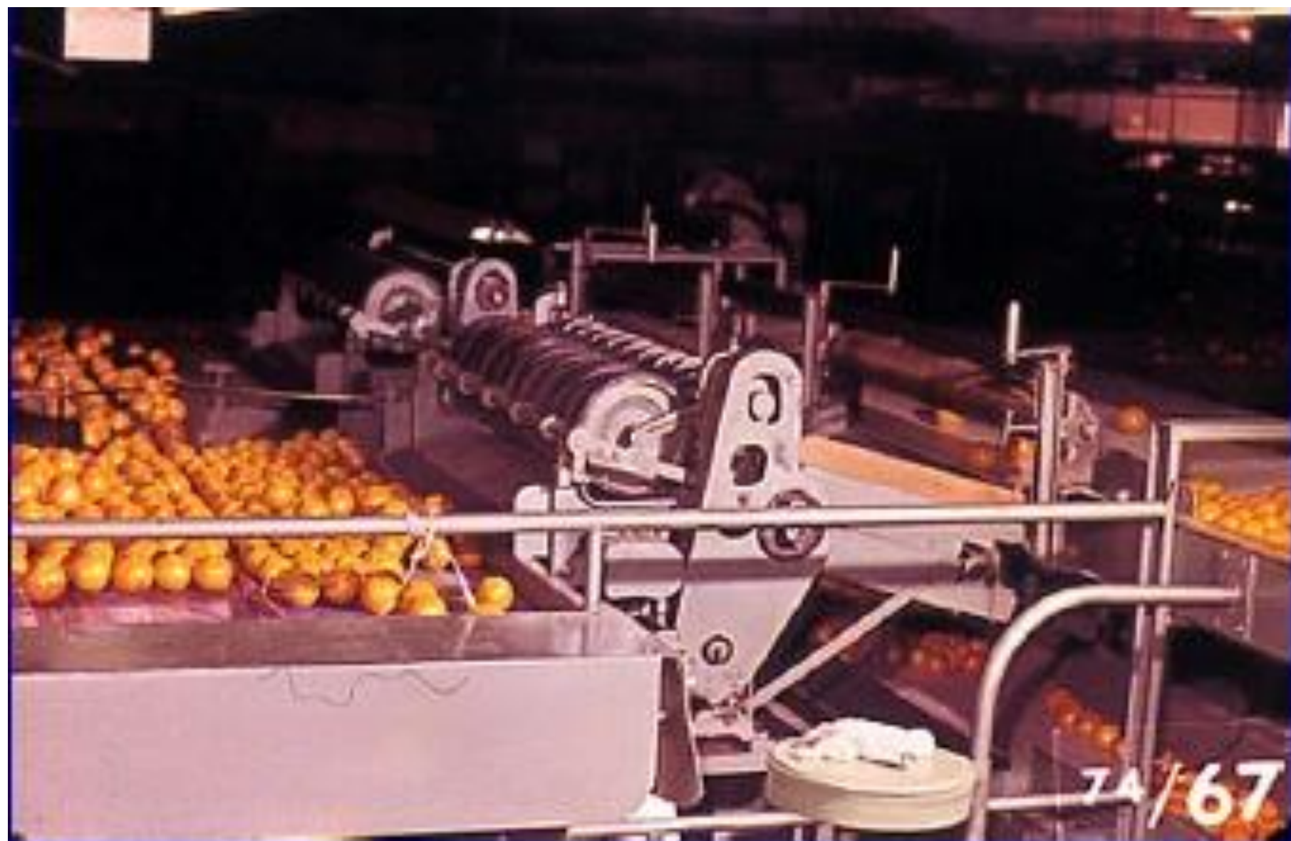
The printing machine which stamps "Sunkist" on each fruit as it passes under the rollers
