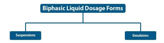
Suspensions are biphasic liquid dosage forms containing essentially insoluble finely divided solid particles or drug(s) suspended with the help of a suspending agent(s) in a liquid medium. The solid particles act as disperse phase whereas liquid acts as a continuous phase.
