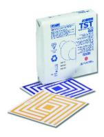
test paper. It consist of standard paper pack and indicator sheet. Sterilizer vacuum performance is acceptable if the sheet inside the test pack shows a uniform color change. Entrapped air will cause a spot to appear on the test sheet, due to the inability of the steam to reach the chemical indicator.
