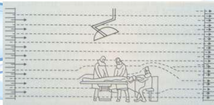
Unidirectional airflow system / lamellar flow ventilation
