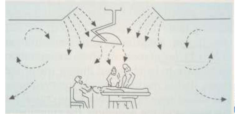
Downward displacement piston system
