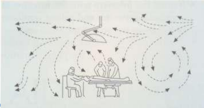
Turbulent / mixing air distribution
