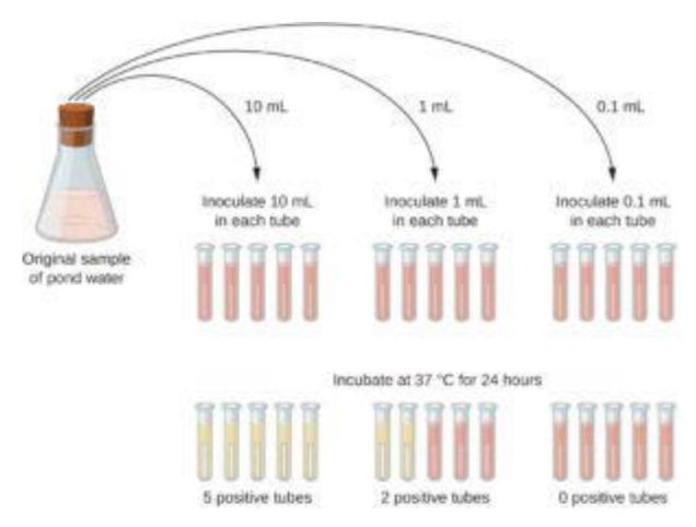
MPN values per 100 ml of sample and 95% confidence limits for various combinations of positive and negative results (when five 10-ml, five 1-ml and five 0.1 ml test portions are used)
