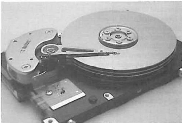
FIGURE 1.7 Computer hard disk drive, showing disks and read/write head
