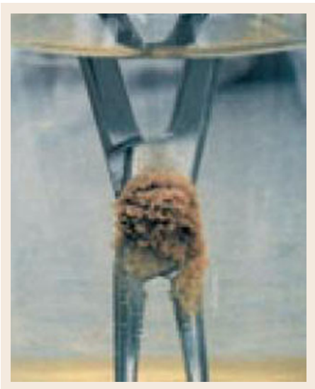
Fig. 72.63 Formation of rust due to multi-hour immersion in physiological saline
