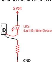
To measure the current going through a simple LED and resistor circuit, for example, you would have to first splice into the circuit somewhere. Here, we spliced into the circuit just after the LED. The current path must go through the meter. Because this is a series circuit, you can measure the current anywhere along this path (i.e. before the LED, after the LED, or after the resistor)
