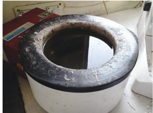
Fig. 5.5 Water bath used in microtomy. The constant temperature (usually 40–50 °C) is maintained in the water bath. This is usually 5–10 °C lower than the melting point of the paraffin
