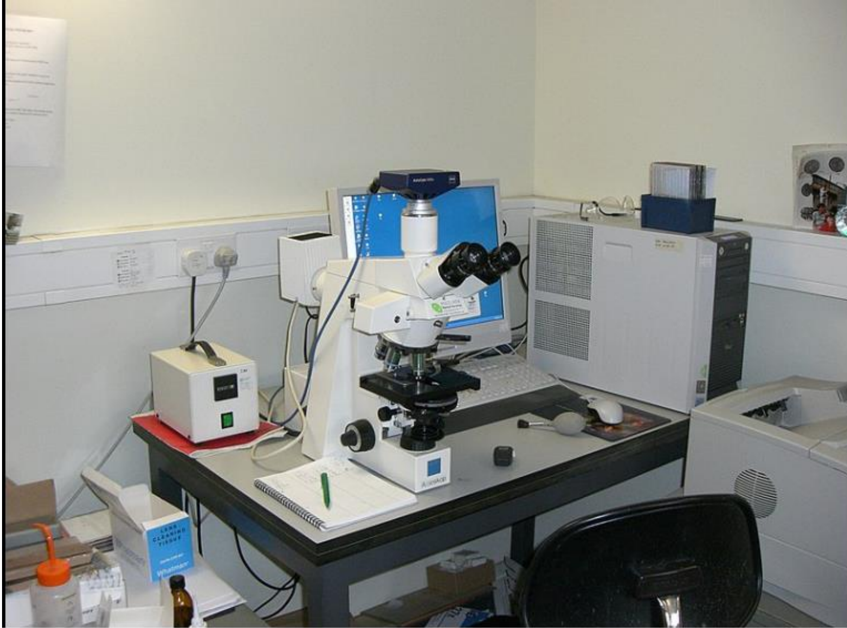
A modern optical microscope with a mercury bulb for fluorescence microscopy . The microscope has a digital camera which is connected to a computer .
