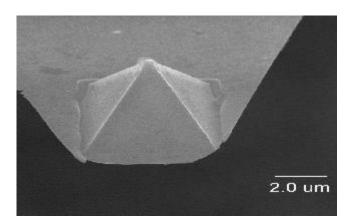
A probe used for atomic force microscopy.
