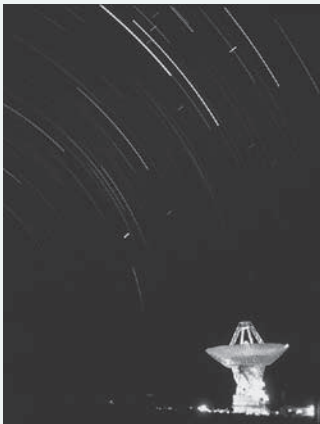
FIGURE 1.8 The search for extraterrestrial life is being carried out with radio antennas like the one pictured here. A radio antenna is an example of a system with position controls.
