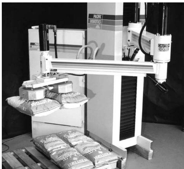
FIGURE P4.11 Vacuum robot lifts two bags of salt.
