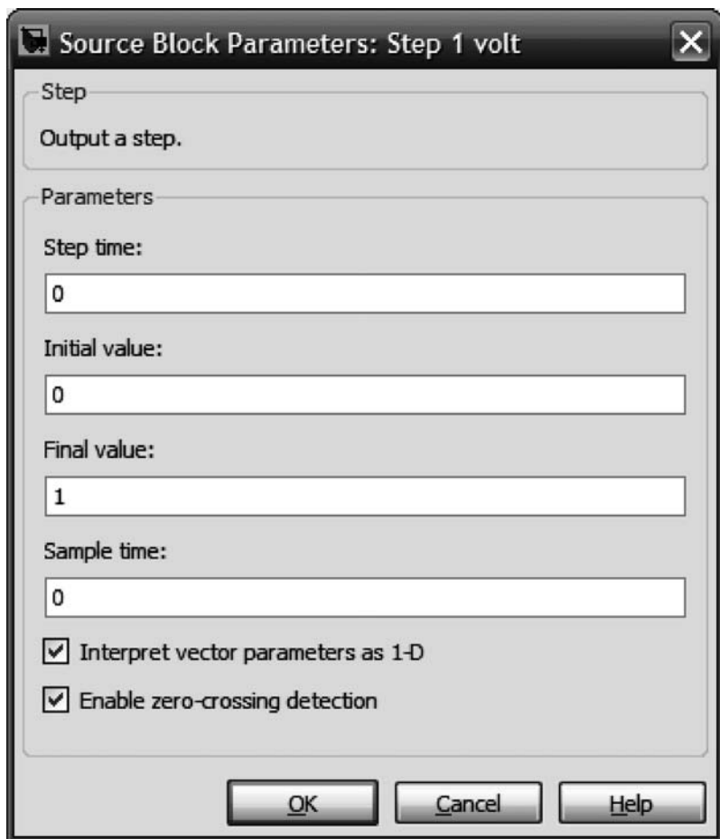
FIGURE C.6 Block parameters windows for a. 1 volt step source; (figure continues)
