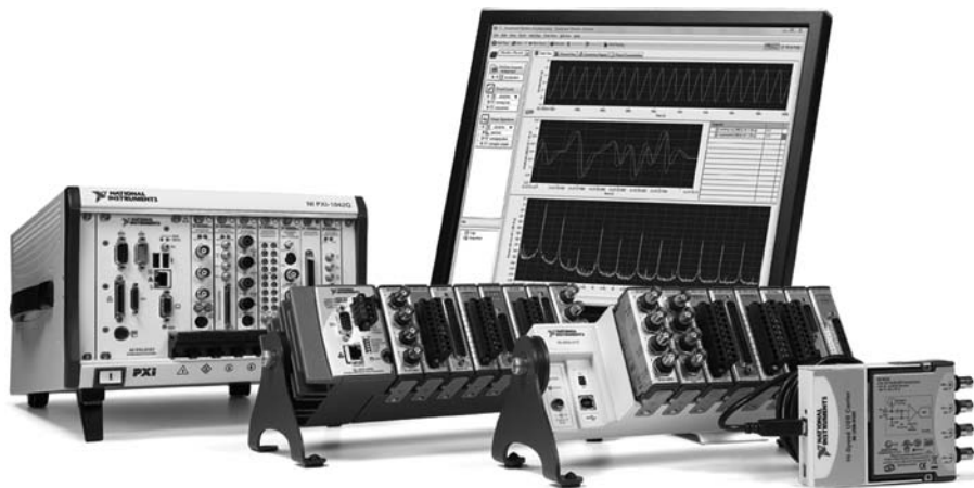
FIGURE 10.1 National Instruments PXI, Compact RIO, Compact DAQ, and USB hardware platforms (shown from left to right) couple with NI LabVIEW software to provide stimulus and acquire signals from physical systems. NI LabVIEW can then be used to analyze data, determine the mathematical model, and prototype and deploy a controller for the physical system (Courtesy National Instruments © 2010).
