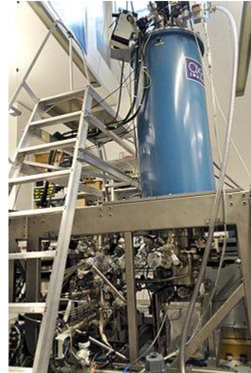
A large scanning tunneling microscope, in the labs of the London Centre for Nanotechnology
