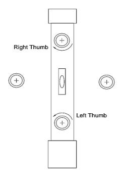
Again, level the telescope using the leveling screws
