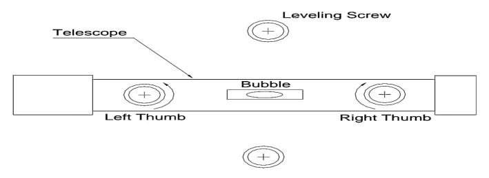
The telescope is leveled by using the thumb and first finger of both hands to adjust the leveling screws until the bubble is approximately centred
