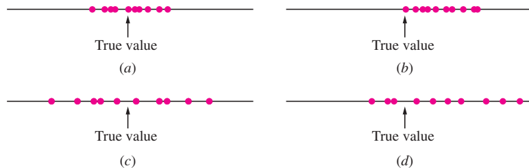
FIGURE 3.1 (a) Both bias and uncertainty are small. (b) Bias is large; uncertainty is small. (c) Bias is small; uncertainty is large. (d) Both bias and uncertainty are large.
