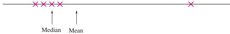
FIGURE 1.3 When a sample contains outliers, the median may be more representative of the sample than the mean is.
