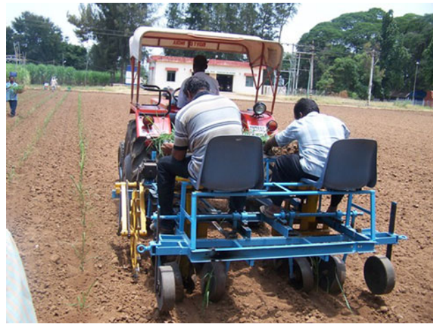
Fig. 7 Field operation of two row tractor drawn mechanical planter for sugarcane bud chip settlings raised in protray (back view) with planted settlings
