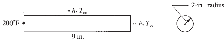
Figure 13–12 One-dimensional rod subjected to temperature variation
