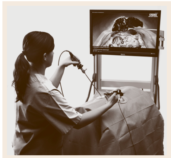
Fig. 19.19 Virtual MIS simulator for laparoscopic interventions
