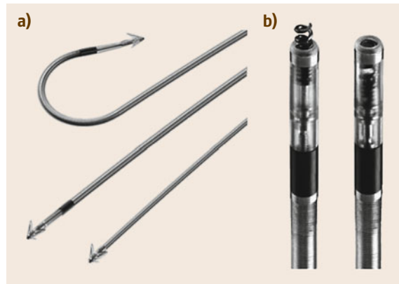
Fig. 38.5a,b Passive (a) and active (b) anchorable probe heads of cardiac pacemaker electrodes. The top passive electrode is a so-called J electrode. Below this follow a bipolar and a unipolar standard electrode. The screw electrode, which must be actively anchored, is shown once with an extended tip (ready for screwing into the myocardium) and, next to this, with a retracted tip (to avoid complications when inserting the electrode in the heart)
