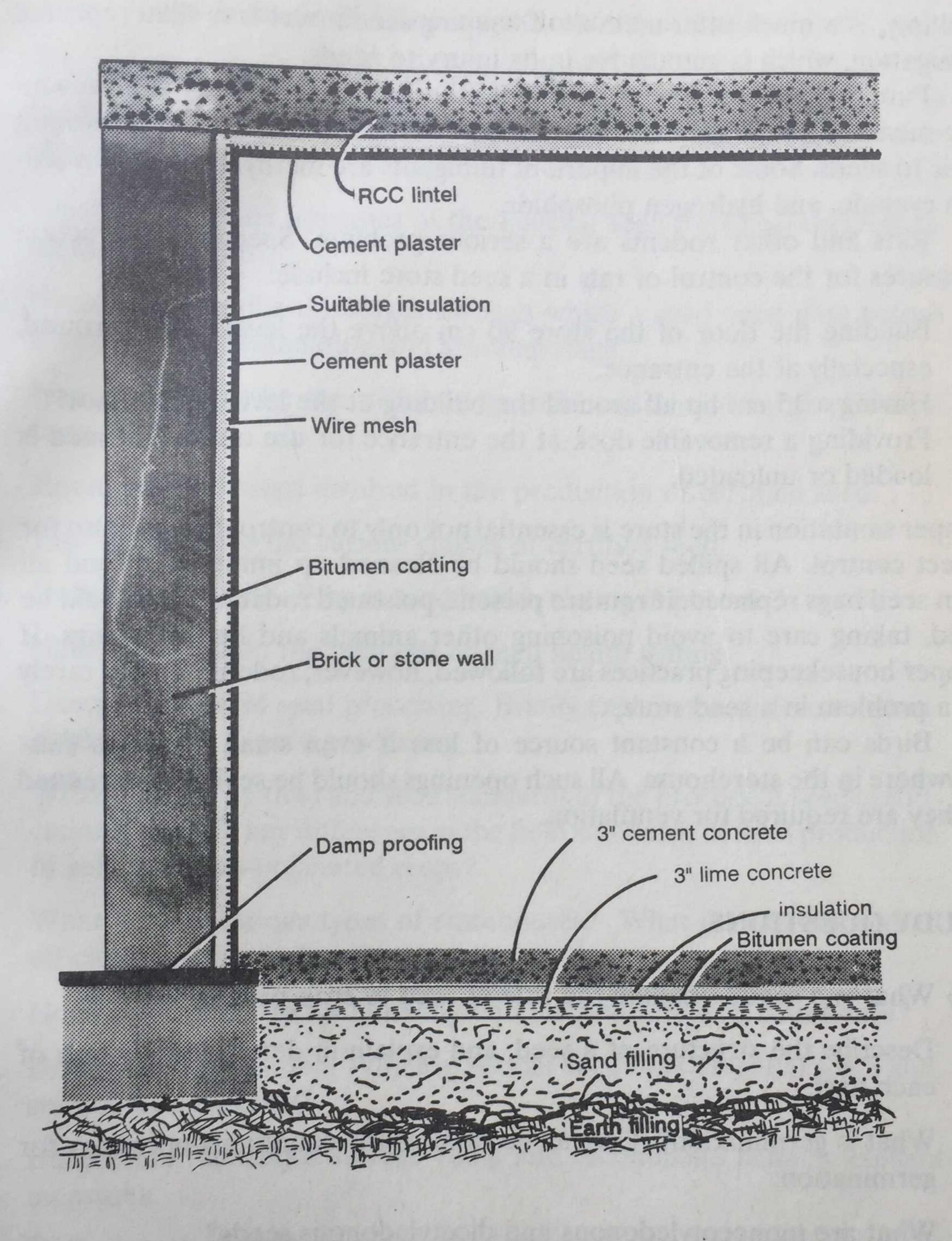
Figure 6.11 Cross-section of a properly insulated and moisture/vapour-proof seed store. Redrawn by Habib-ul-Rahman Mian following Feistritzer 1975a.
