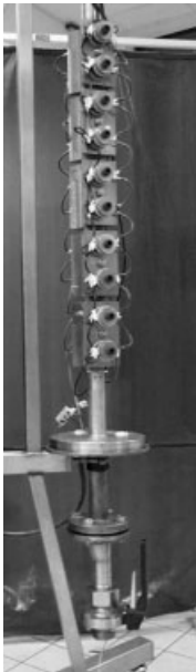
Fig. 7.5 Example of a radially vibrating system from Sonic Process Technologies.
