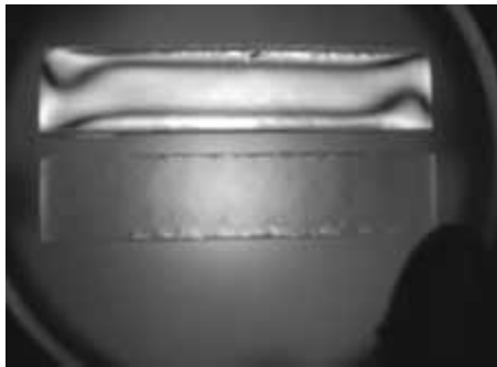
Figure 22.17 Annealing a solid allows the atoms or molecules to adopt a different, more stable structure. The first picture shows the solid (glass) before annealing, and the second picture shows the same solid after annealing.
