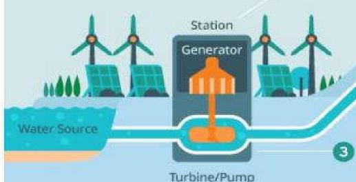
Renewable energy such as wind or solar used to pump water uphill during times of low demand
