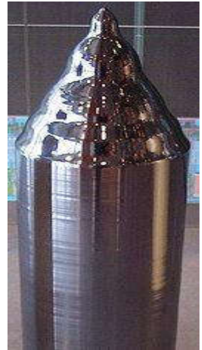
Si boule for the production of wafers.
