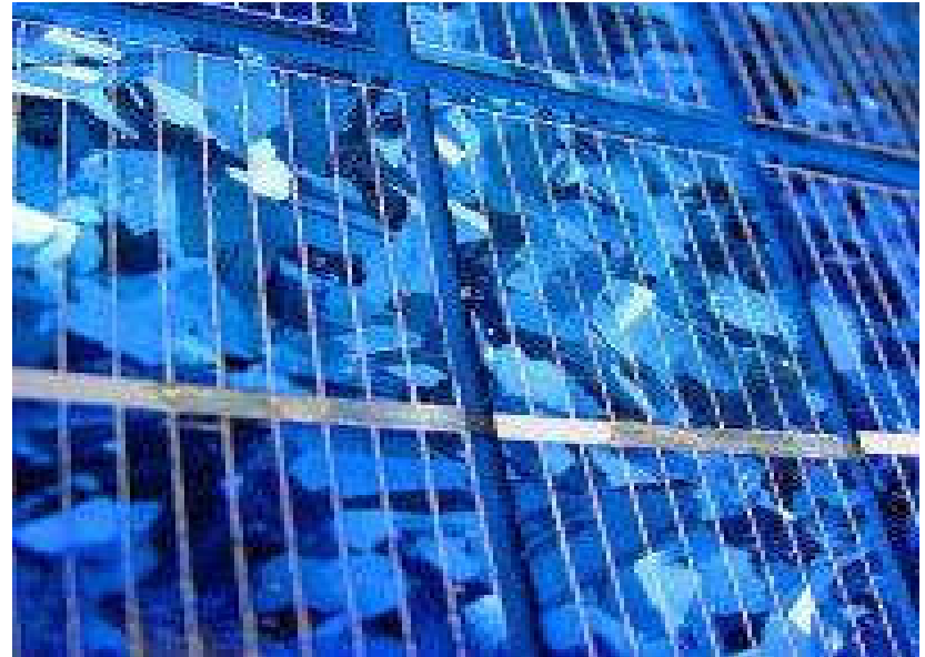
Visible crystal grain in poly-Si
