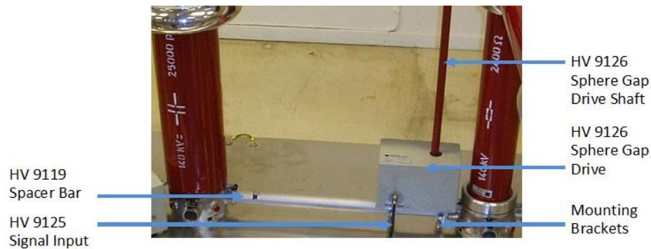
Fig. 8.7 HV 9126 Sphere Gap Drive Placement
