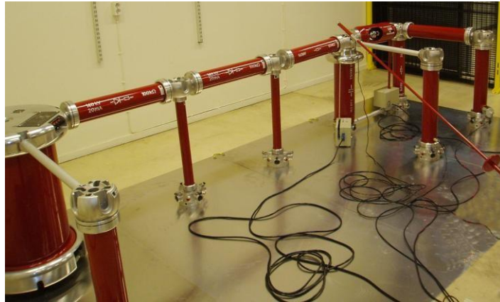
Fig 8.10 Impulse Setup almost complete - Cables to be organized
