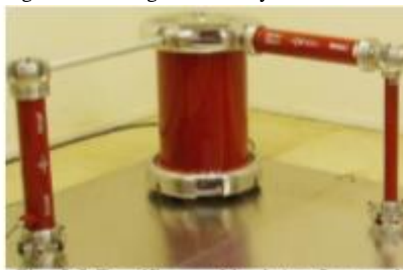
Fig 4.4 Rectifier and Isolator secured
