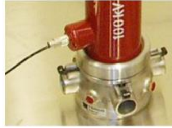
Fig 2.10 AC Measuring Capacitor output
