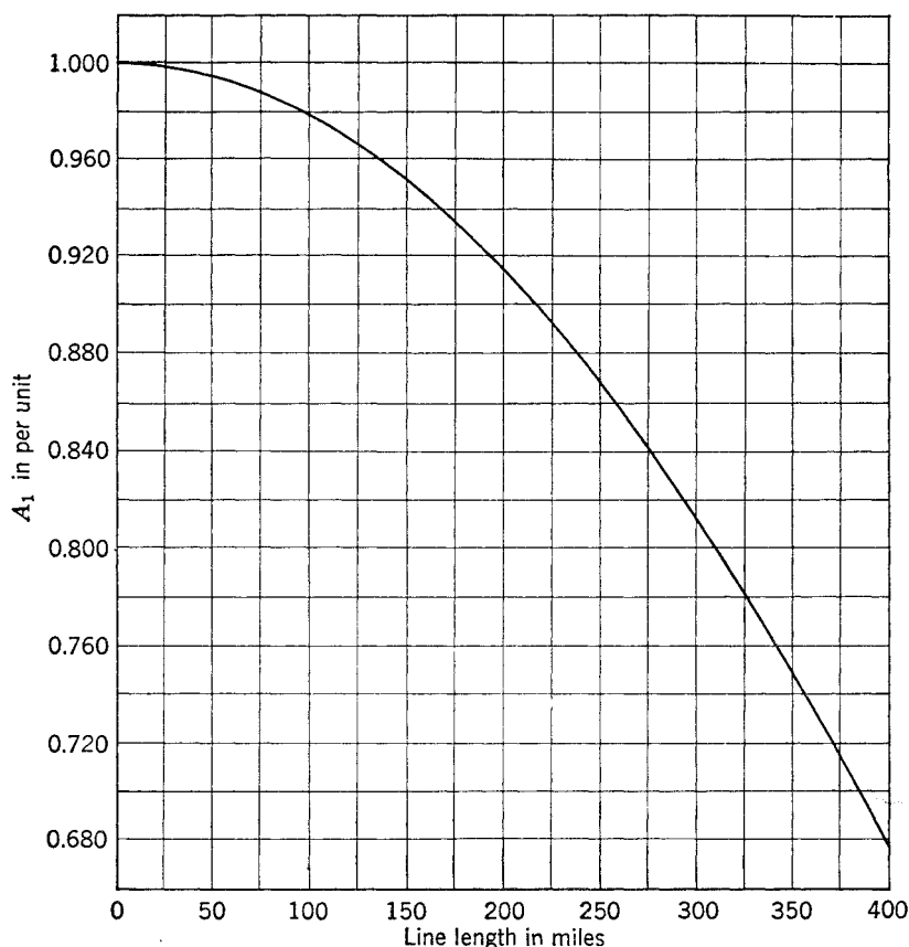
FIG. 6.7 The transmission-line A_1 constant as a function of line length in miles. (From D. J. Povejsil and A. A. Johnson, "A Per-unit Interpretation of Transmission Line Constants," Trans. AIEE , vol. 70, pp. 194-200, 1951, by permission.)
