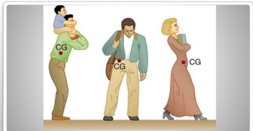
Comparison of Factors Affecting Location of Center of Gravity in the Human Body Relative to Load being Carried
