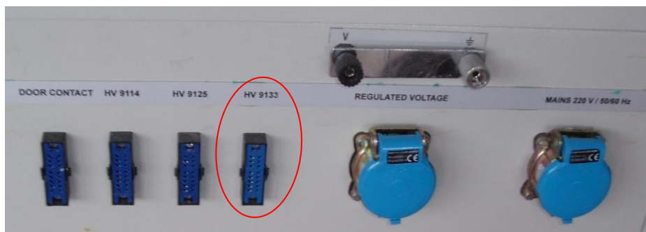
Fig 3.7 HV 9133 Sphere Gap Motor Control Input
