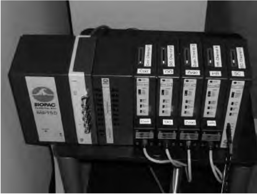
Figure 7.4 The Primary Component for Psychophysiological Data Collection consists of a Configuration of Bioamplifiers and a Skin Coupler like Shown Here. The equipment shown here is used for the collection of peripheral nervous system measures (heart rate, skin conductance, and facial EMG).
