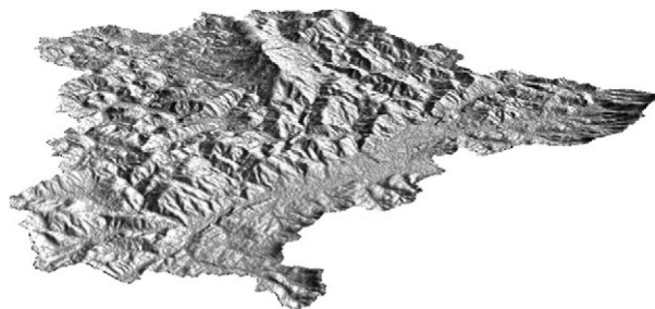
Figure 8 One meter digital elevation model generated from LiDAR data with an average point spacing of approximately 5 m. ESRI terrain dataset generated from original bare-earth LiDAR points from the North Carolina Floodplain Mapping Program. The 1 m DEM was created to enhance hydrographic modeling operations within the watershed. DEM courtesy of Jeffrey Colby, Appalachian State University.
