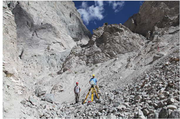
Figure 1 Terrestrial laser scanning at the Chalk Cliffs Natural Debris Flow Laboratory (Summer 2010). A Leica HDS C10 laser scanner was used for repeat surveying. Pictured in the image are Thad Wasklewicz (yellow helmet) and Dennis Staley (red helmet). Photograph courtesy of Thad Wasklewicz, East Carolina University.
