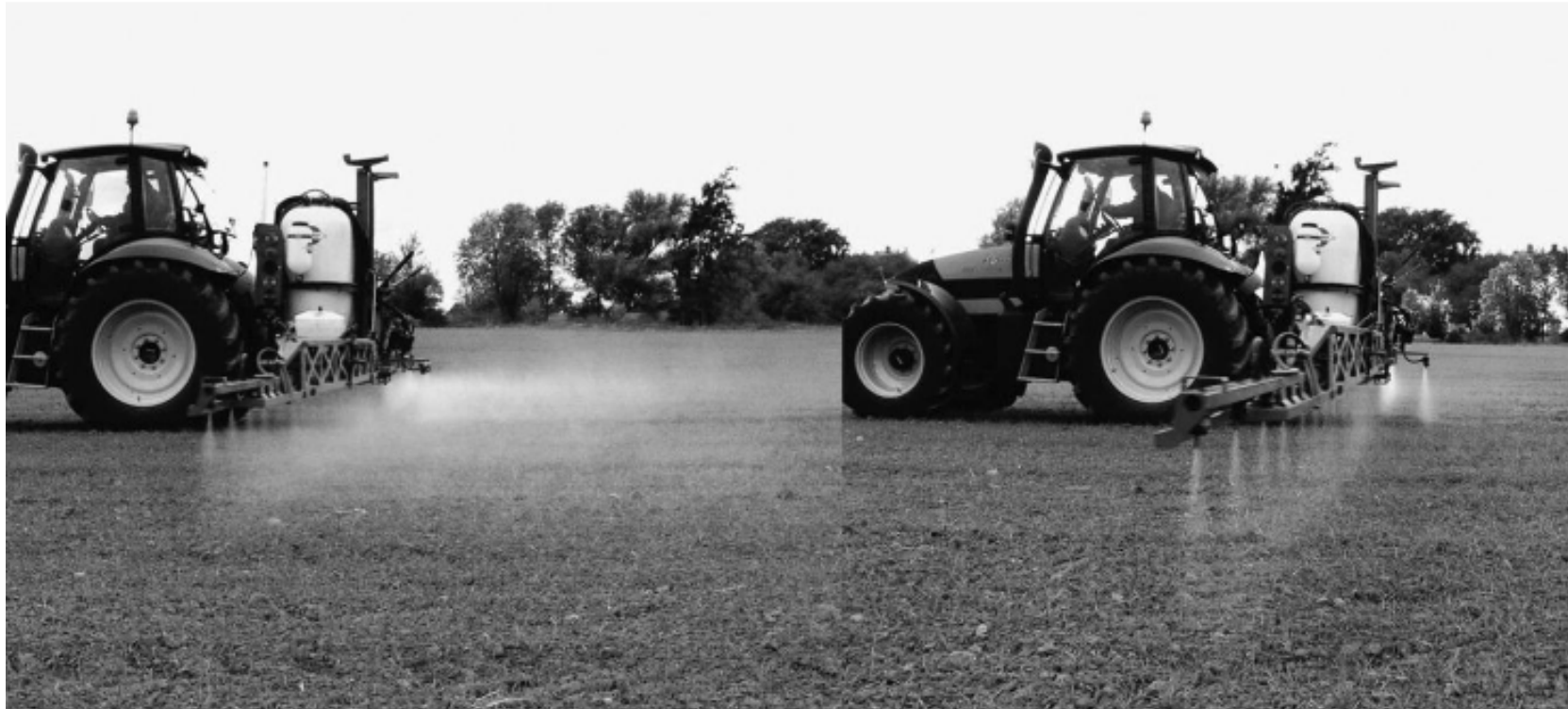
Fig. 6.6 Comparison of spray drift with conventional flat fan nozzle and reducing drift with different nozzle (Photographs courtesy of Hardi International).
