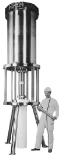
FIGURE 22-8 Industrial-scale preparative chromatography column can purify a kilogram of material. The column volume is 500 L. [Courtesy Prochrom, Inc., Indianapolis, IN]
