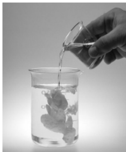
FIGURE 6-2 A yellow solid, lead(II) iodide ( \text{PbI}_2 ), precipitates when a colorless solution of lead nitrate ( \text{Pb}(\text{NO}_3)_2 ) is added to a colorless solution of potassium iodide ( \text{KI} ). [Photo by Chip Clark.]
