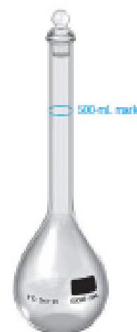
FIGURE 1-3 A volumetric flask contains a specified volume when the liquid level is adjusted to the middle of the mark in the thin neck of the flask. Use of this flask is described in Section 2-5.
