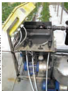
Plate 14 Open mixing tank that allows completion of the acid/bicarbonate reaction
