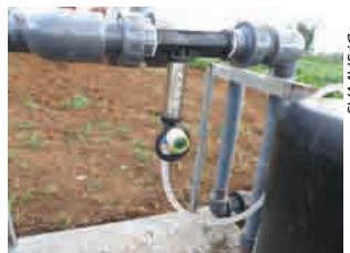
Plate 13 Venturi device as part of a simple volumetric injector used to prepare nutrient solution by diluting stock solutions with water
