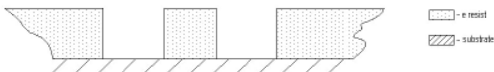
Fig. 2.3. E-resist crosssection: Only the chemically changed e-resist can be dissolved in the specific solvent (positive lithography)
